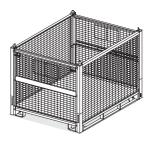
The maximum weight for a loaded ULD is 600kg (including the weight of the ULD which weigh around 100kg). This means that 500kg is available for the contents. Be aware that ULDs will often exceed the maximum weight limit before they are completely full. In order to maximise transportation efficiency and ULD utilisation, you should ensure that each ULD is used as efficiently as possible.
